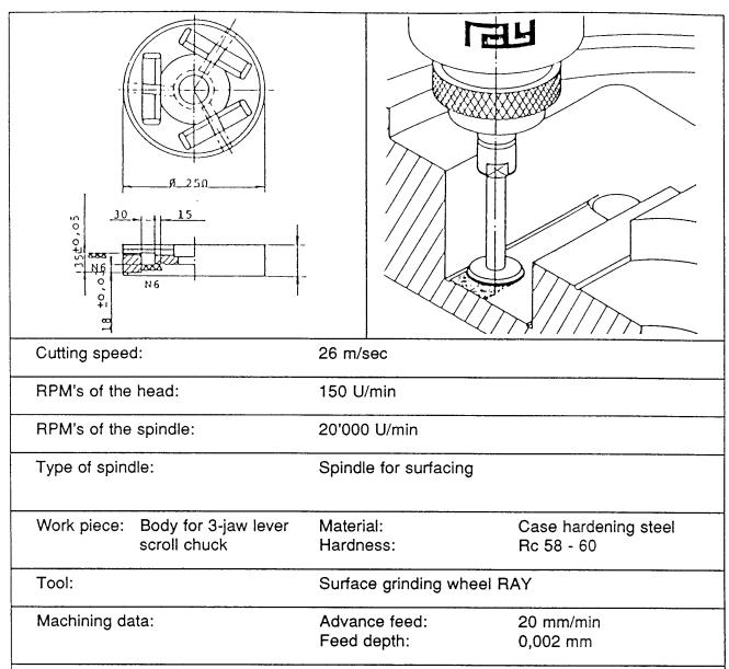
Surface grinding of the base plates of a 3-jaw lever scroll chuck.
