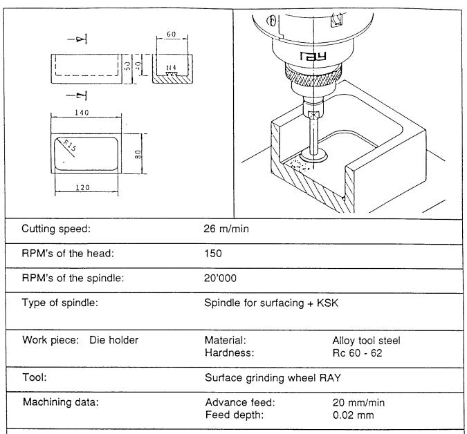
Surfacing of a die holder, which will lateron have to hold the respective tools. The surface will therefore have to be absolutely flat.
