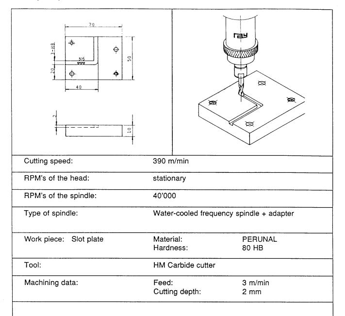
Water-cooled RAY high frequency spindles, used on a milling machine for machining slots in aluminum.
