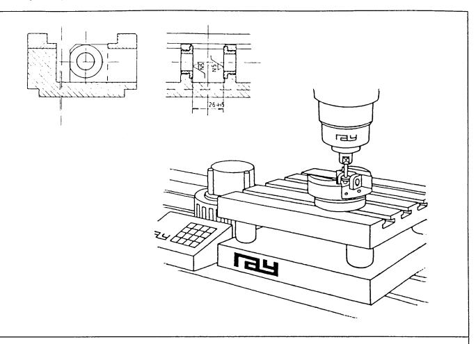
In this working study we have to grind a slot 26H5. For technical reasons it is not possible to use a surface grinding machine or the KSK.
