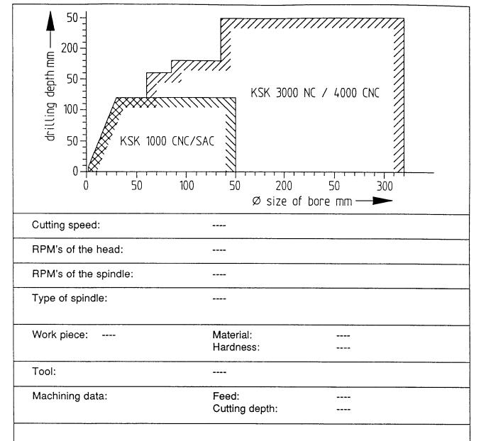
Since almost all of the RAY high frequency spindles can be equipped with grinding pins, the maximum machining depth depends on the spindle and the corresponding grinding pin being used.
