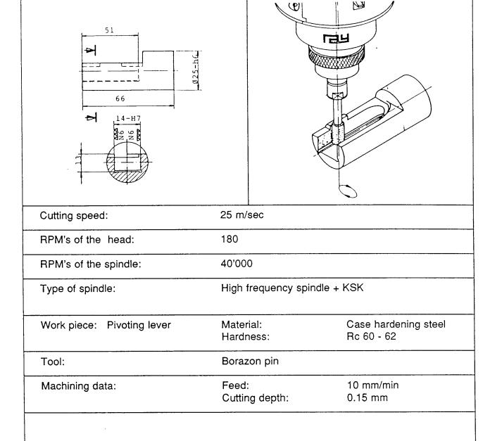
Here a slot 14H7, with a depth of 13 mm is being ground with the KSK.
