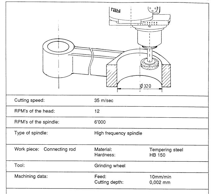
For large bores the rpm of the spindle is the most essential factor. We are working here with grinding wheels.
