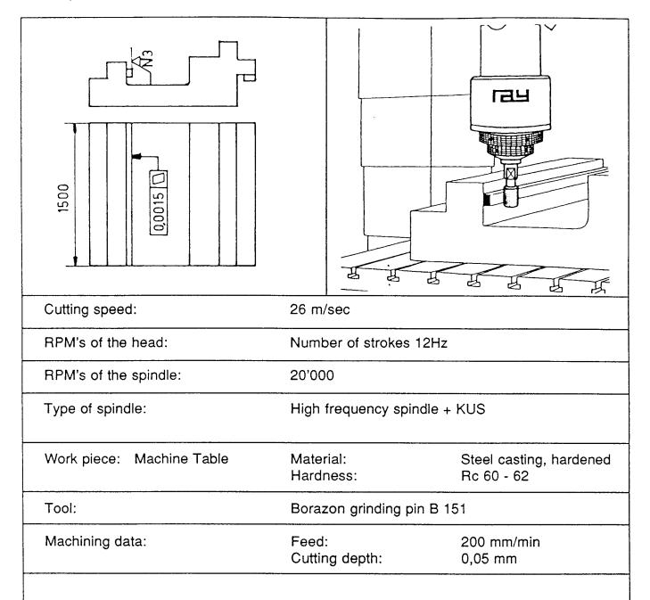
With the cam grinding head KUS a hardened guide rail, which is mounted onto a machine table, is being finish round.
