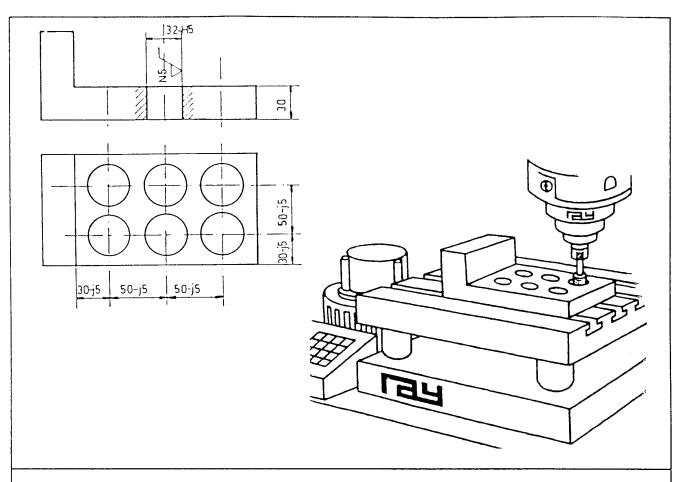
With the HUB the internal grinding with the KSK has been tremendously simplified, since the oscillating movement has been taken over by the HUB.
