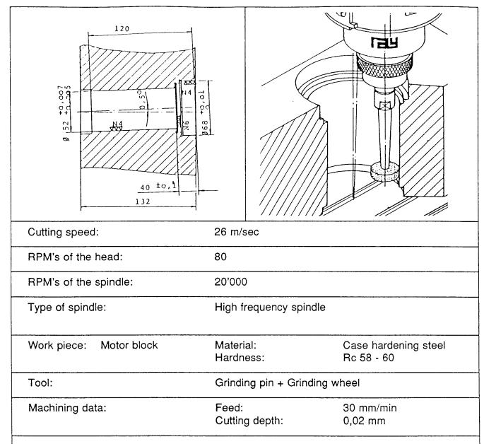
Here we are working vertically with a grinding pin and a grinding wheel.
