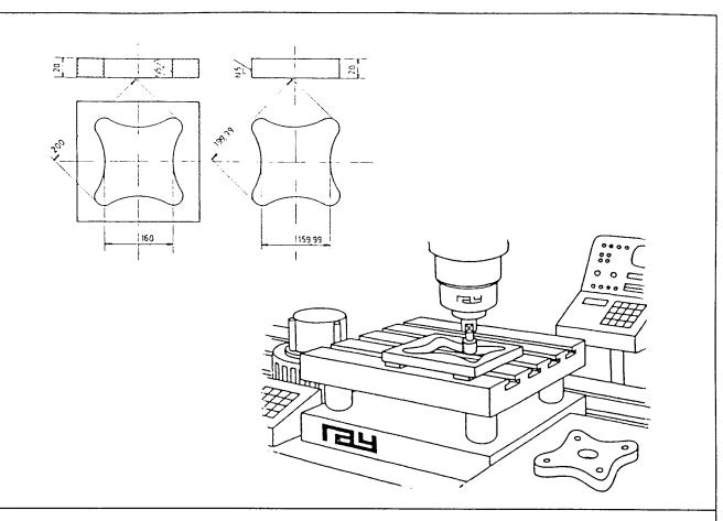
For the grinding of this stamping die the HUB is a MUST. In order to obtain a die clearance of 0,01 mm, a cylindricity of minimum 0,004 of the die, respectively of the die plate, is required. This, however, necessitates on the other hand that when finishing, the grinding wheel protrudes from the work piece, i.e. it will have to move over the entire grinding surface.
