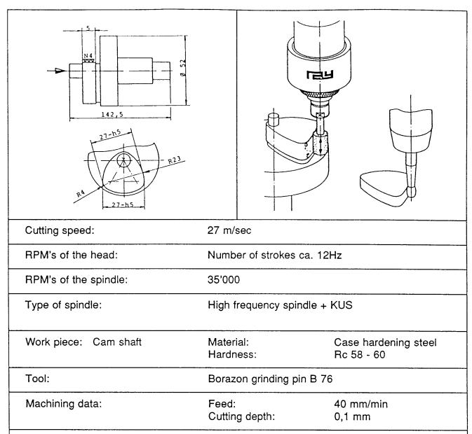
Grinding of the cam of a cam shaft with the KUS on a copy milling machine.
