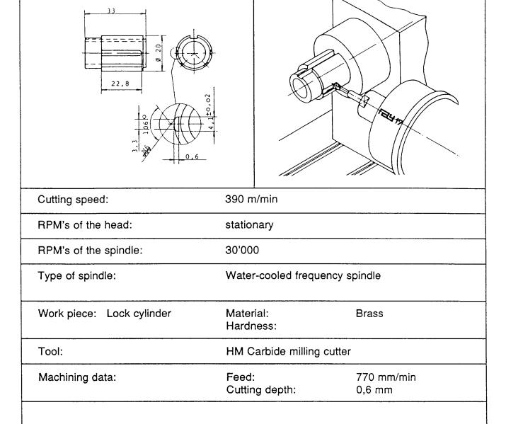
With a stationary, water-cooled RAY spindle and a single purpose machine, dovetail slots are being milled into a lock cylinder.
