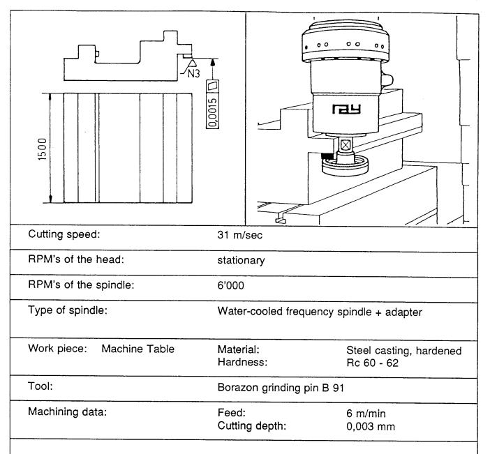
By means of a stationary, water-cooled RAY spindle, which was mounted onto a machine table, a hardened guide rail had to be finish ground.
