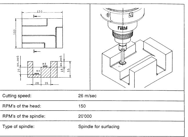
Tool: Surface grinding wheel RAY
