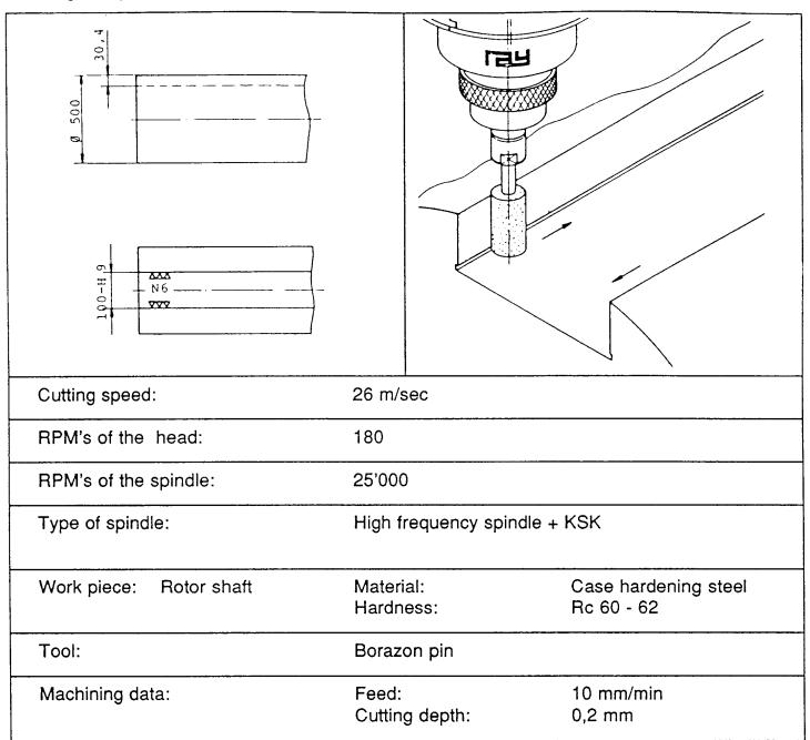
In this example a larger slot is being ground with the KSK, whereby first one side and then the other side is being machined.
