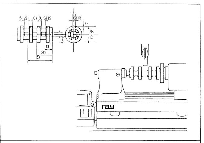
In this study the oscillating apparatus is used for the slotting work of keyways.
