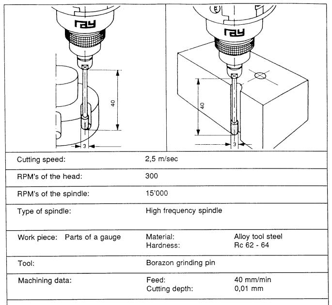
According to the optimum circumferential speed for Borazon, this grinding pin could turn at approx. 60'000 rpm or more. It is evident that this is not possible for safety reasons.
