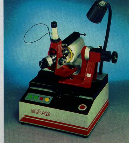
Execution for printed circuit board drills Meteor MM-10-PD
