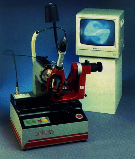
Execution with camera-monitor Meteor MM-12-TV
